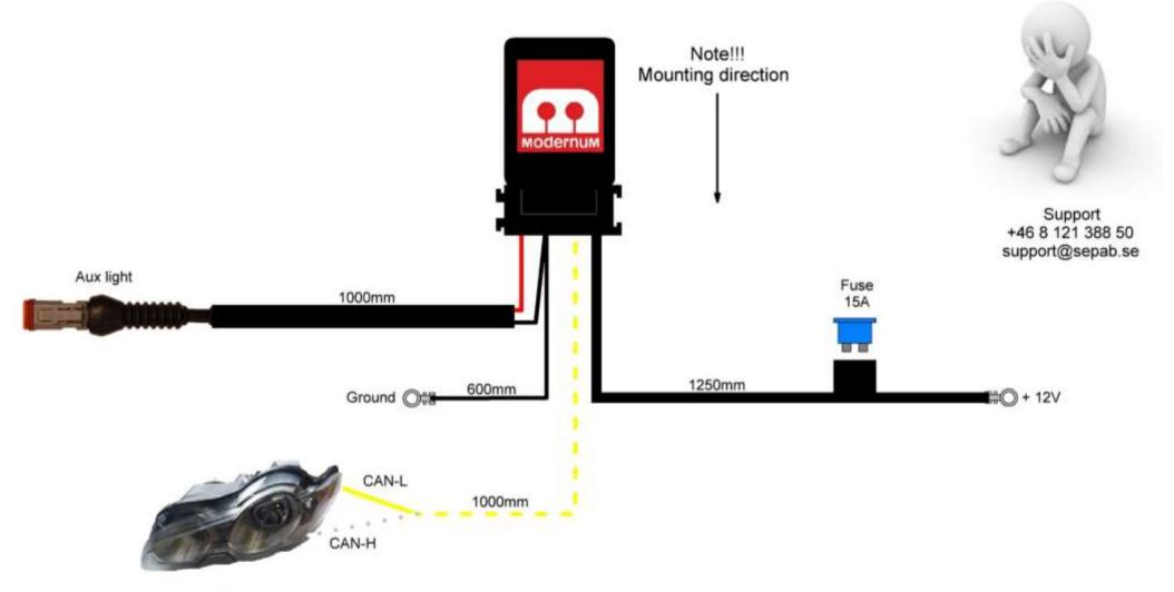
Note! White (CAN-H) and yellow (CAN-L) twisted cable = Digital signal in.
