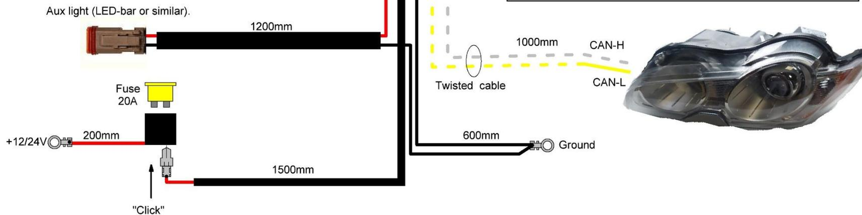
*NOTE! White (CAN-H) and yellow (CAN-L) twisted cable = Digital signals in.*
