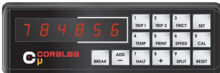
To calibrate temperature, place the sensor into ice water. Ice water has a known temperature of 32 degrees Fahrenheit or 0 degrees Celsius. Next, follow the calibration steps listed below:
